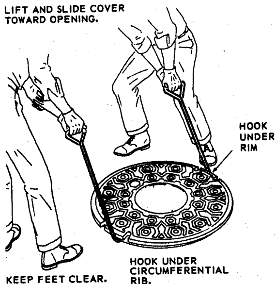
Figure 9. Moving Cover Along Ground.
